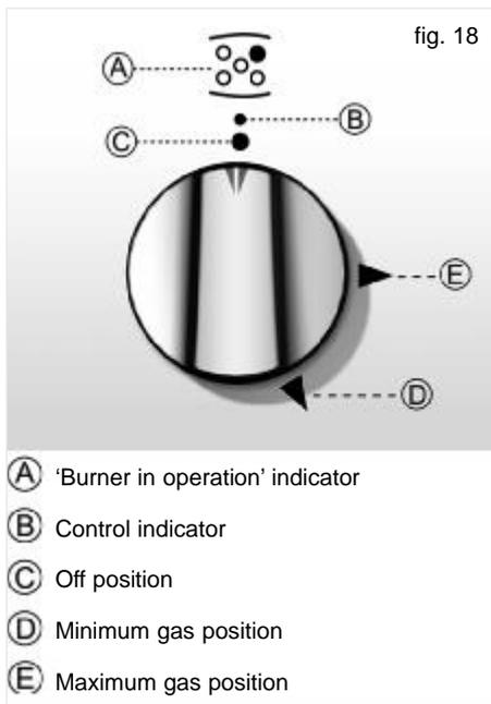
**With hobs CG Lux-60, CG Lux-70, CG Lux-75, CG Lux-86 and VR 90 4G, which have automatic ignition and safety, proceed as follows:** (See fig. 19)
