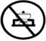
Do not use small pans on large burners, or the flame will spread.
